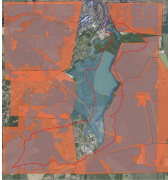
Fig. 4 Based on a GIS analysis, large areas in the Regenbeek catchment were excluded for building a rain storage reservoir
